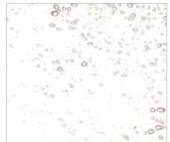
polyalphaolefin (PAO) air release: 12 seconds
