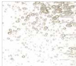
gas-to-liquid (GTL) air release: 15 seconds
